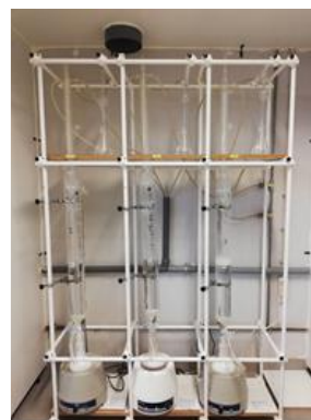
Figure 1. Perforator apparatus – EN ISO 12460-5.
