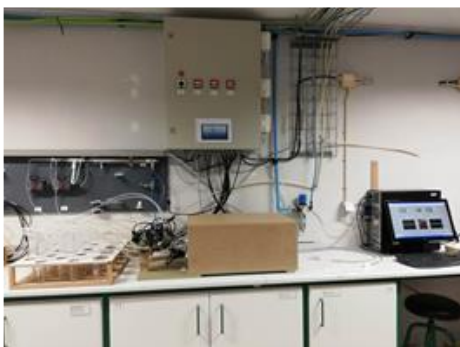
Figure 2. Gas analysis chamber – EN ISO 12460-3.
