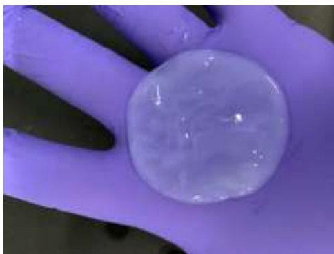
Figure 1. Hydrated BC membrane collected immediately after production by K. Rhaeticus , a non-pathogenic Gram-negative bacteria of the genus Komagateibacter .
