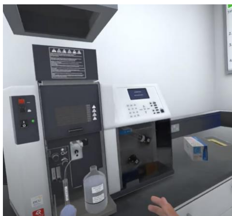
Figure: Screen grab of virtual AAS instrumentation from the Immersive Chemistry Lab hosted on Meta's AppLab.
