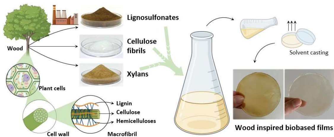
Figure 1: Schematic illustration of the preparation of the films.
