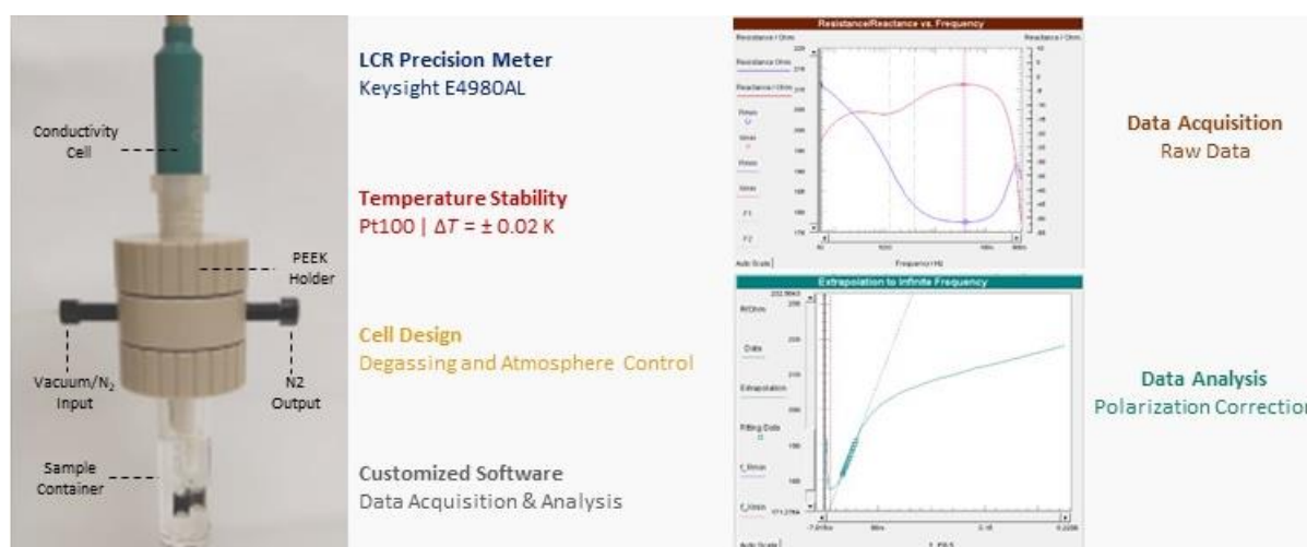
Figure 1. Representation of the measuring system and data treatment.
