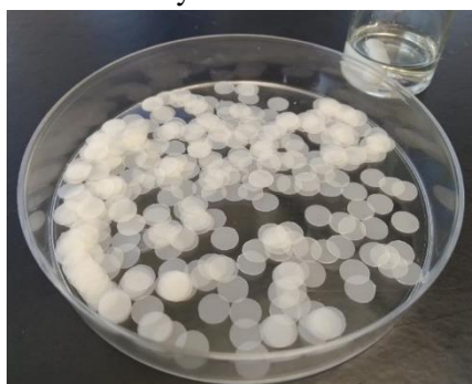
Figure 1. PVDF membranes impregnated with NADE.
