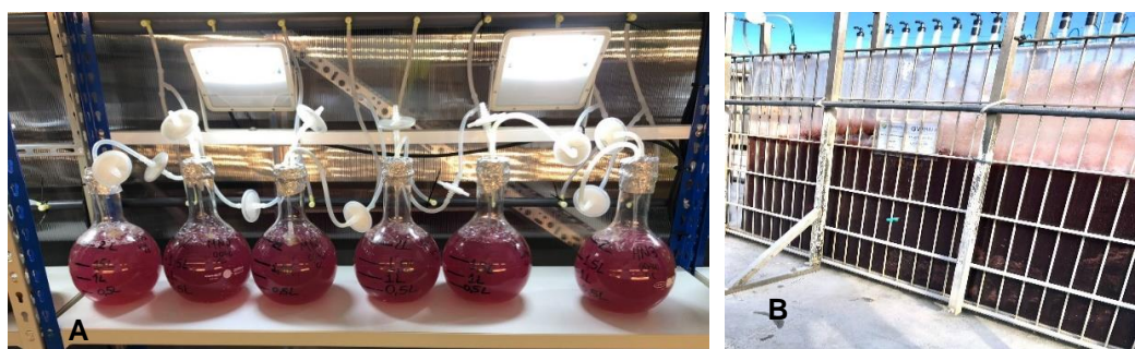
Figure 1. Growth of P. cruentum cultures in (A) lab scale and (B) flat panel photobioreactors.
