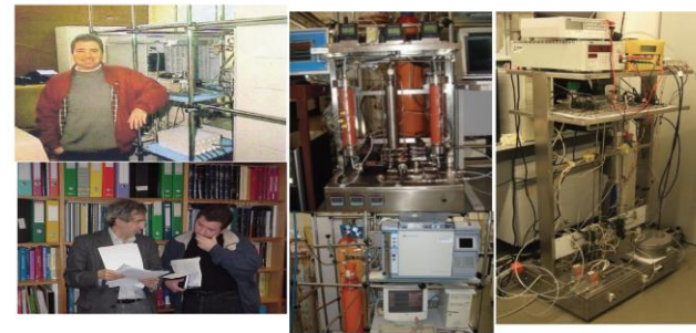
Lab-scale PSA units :single column unit and 2-bed PSA. Electric Swing Adsorption
