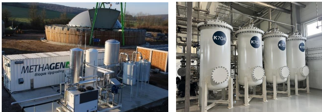
Image 2. (Left) METHAGEN AD for agricultural waste biogas in Premery, France: biomethane for grid injection; (right) METHAGEN AD upgrading biogas produced from chicken manure in Iecava, Latvia: biomethane for grid injection.
