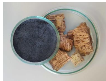
Image 1. A black carbon material produced through the pyrolysis of cork
