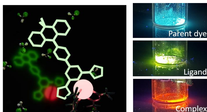
Figure. Left: schematic representation of a lanthanide complex. Right: pictures of luminescent powders of TADF dyes under 365 nm irradiation.
