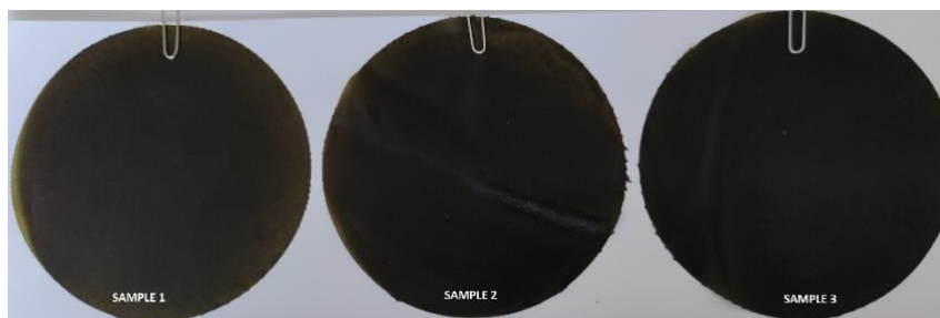
Fig.1. SuOC biopolymer films with different thickness (trend of increasing thickness from left to the right)
