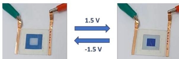
Figure 1: ECSC prepared with PEDOT:PSS as electrode material and gel polymer electrolyte.
