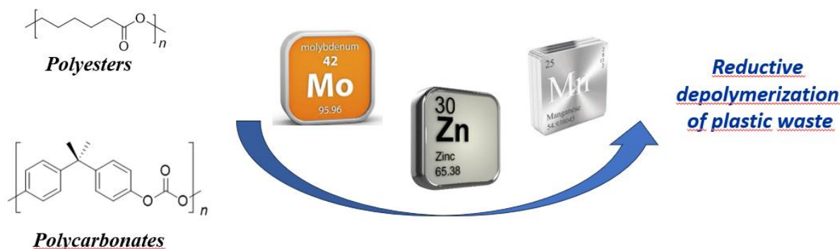
Figure 1: Reductive depolymerization of plastic waste catalyzed by molybdenum, zinc and manganese compounds.
